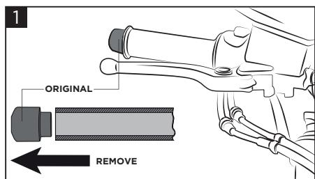
**Untighten the original screw and remove the counterweight.**
