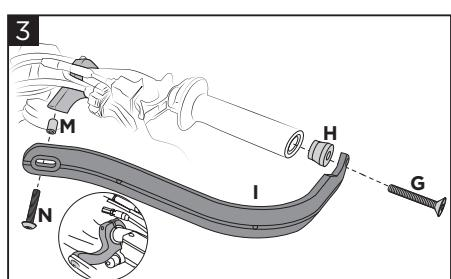
**Fix the bar (I) to the handlebar using the spacer (H) and the screw (G) as shown in the figure. Fix the bar to the bracket using the bushing (M) and the screw (N).**
