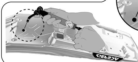
**To inflate the internal bladder connect the included needle tip to the pump and insert into the seat. For best results lube the needle with a silicone based lubricant.**
