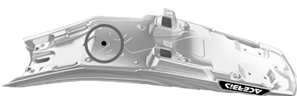
**The inflation valve is located under the seat. A manual hand pump is required to inflate the seat.**
