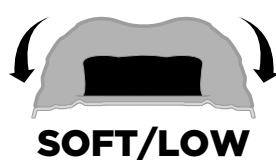
**The firmness/height of the seat changes based on how much pressure is in the internal bladder.**
